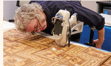
FIG 2. Fran Baas conducts an X-ray fluorescence test on metal fragments stuck to an ancient painted textile from the John and Nora Wise Collection, 1983.W.1915. Photo by Brad Flowers.
